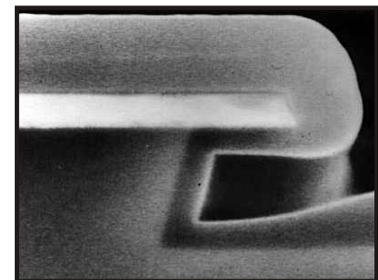
2 µm SiO<sub>2</sub> deposited over a test structure
