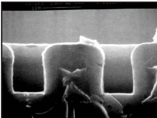
250 nm SiO<sub>2</sub> deposited over 1 µm wide lines
