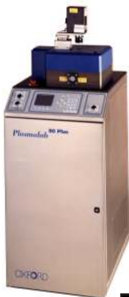
Plasma Enhanced Chemical Vapour Deposition (PECVD)
