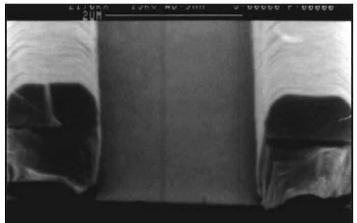
OPT application lab: 1.5 \mu\text{m} deep Al/Si etch (PR mask in place)
